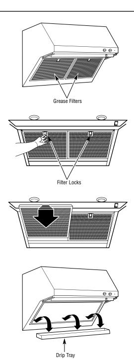
Baffle grease filters and drip trays (on some models)
