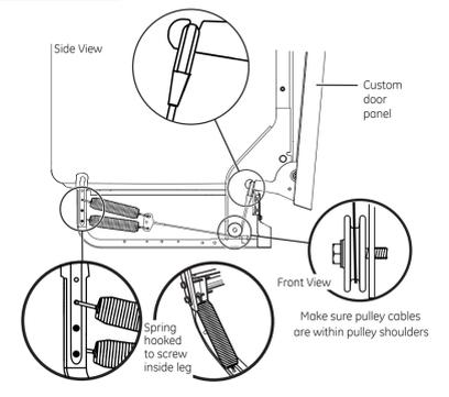
**TIP:** If the door does not open easily or falls too quickly, check spring cable routing. The cable is held in place by "shoulders" on the pulley. Check to be sure the cable has not slipped over the pulley shoulders.
